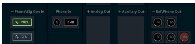
Routing to the analog output (optionally to Dante out if going to a Dante enabled unit) and to a reference channels.
