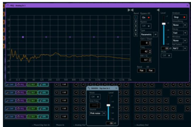
The room measurement (below) has three primary areas of interest to achieve a flat response that's approximated by the horizontal pale green line as the target; this line is a graphic overlay for clarity and is not part of the tool. Reading left to right the first area of interest is the low frequency end of the scale that is outside of the speech range but is definitely in the mechanical noise range. We don't want to pick up this noise so we apply a sharp **Low Cut** filter.
