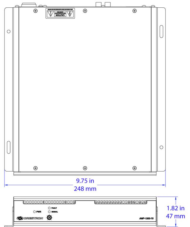
Unit with surface mounting kit installed
