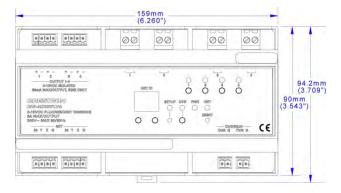
The DIN-4DIMFLV4 is a 4-channel lighting control module designed to support dimming of 4-wire 0-10 volt fluorescent dimming ballasts. A single model supports both 120 and 220-240 volt applications. Each channel handles up to 30 dimmable ballasts, and may also be used for switching of non-dimmable lighting loads up to 5 amps, as well as 1/2 HP motors.
