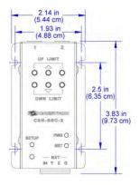
The C2N-SSC-2 Somfy Shade Controller is a compact Cresnet device designed to provide a bidirectional serial interface for up to two Somfy ILT Intelligent Shade Motors (http://www.somfy.com/nam/index.cfm). Window treatments equipped with the Somfy ILT motor offer enhanced capability compared to typical 3-wire models.
