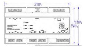
The DIN-AP2 is a 2-Series control processor designed for small to medium-sized lighting and automation applications. DIN Rail mounting enables modular installation alongside Crestron DIN Rail lighting and automation control modules and other third-party DIN Rail mountable devices.
