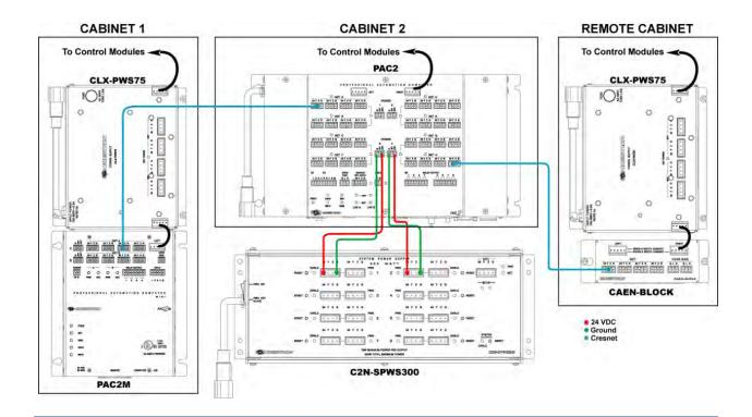
**NOTE:** If more than 50 watts of power is drawn by connected devices, supplemental power supplies are required.
