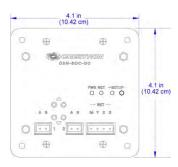
The C2N-SDC-DC is a 2-channel shade and drape controller designed to provide a convenient and cost-effective solution for controlling 24 volt DC motorized shades and drapes. The C2N-SDC-DC is a Cresnet device with two independently controlled 24V DC outputs, each designed to provide standard up/down or open/close control of a conventional two-wire bidirectional type motor.
