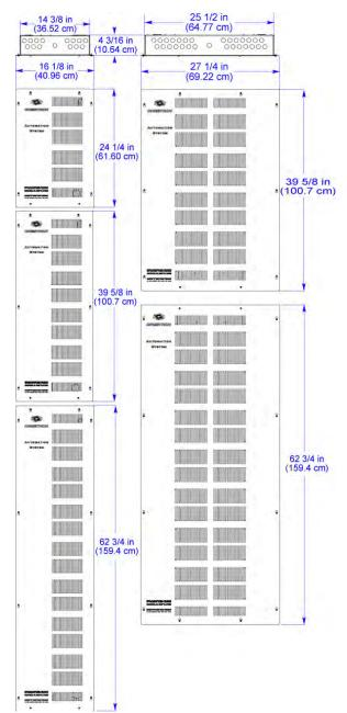
The CAEN Series automation enclosures are designed to house the Crestron CLX-series of lighting and motor control modules and PAC2 or PAC2M control systems. CAEN enclosures are available in an assortment of sizes, suitable for surface or flush wall mount installation. Each model has been engineered to provide a clean and manageable installation with abundant provisions for wire termination and electrical knockouts.
