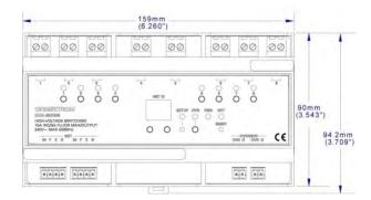
The DIN-8SW8 is an 8-channel high voltage lighting control module designed to support switching of non-dimmable lighting and fans. A single model supports both 120 and 220-240 volt applications. Each channel handles incandescent loads up to 10 amps, fluorescent loads up to 5 amps, and also 1/2 HP motors.
