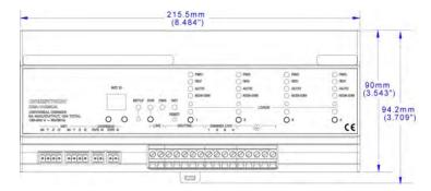
The DIN-1DIMU4 is a 4-channel universal lighting control module designed to support dimming of both forward and reverse phase type loads. A single model supports 120 and 220-240 volt electronic and magnetic low voltage, incandescent, neon/cold cathode, 2-wire dimmable fluorescent, and non-dimmable lighting loads up to 5 amps per channel, 10 amps total.
