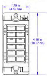
Crestron C2N-DB Decorator Series keypads deliver versatile keypad control with contemporary styling to support a broad range of residential and commercial applications from lighting to AV distribution.
