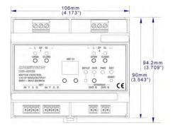
The DIN-2MC2 is a 2-channel motor control module designed to provide control of bidirectional motors for drapes, shades, projection screens, lifts, skylights, and gates. Each channel supports up/down or open/close control of a conventional 3-wire bidirectional type motor up to 1/2 HP at voltages up to 240 volts. Built-in timing and interlock logic make it easy to program the DIN-2MC2 for failsafe operation.
