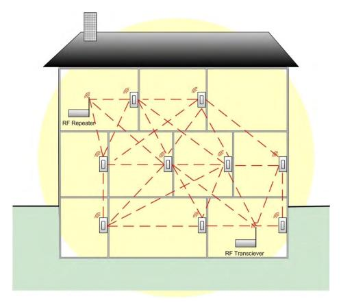
Crestron infiNET Wireless System
