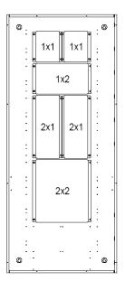
Crestron Universal Mounting Plates (CAEN-UMP Series) are a complete line of accessory plates, which allow mounting of non-Crestron equipment to any Crestron Automation Enclosure (CAEN Series). Third-party products such as phone and alarm systems can be mounted to these plates. The advantage to using the CAEN-UMP is that a variety of sizes are available and each plate occupies the same area as one, two or four Crestron lighting modules (CLX-series).
