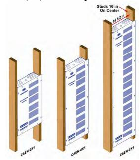
allow adequate clearance in front of the vented cover for servicing and ventilation.
