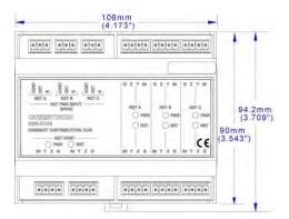
The DIN-HUB is a DIN Rail-mounted Cresnet® hub designed to facilitate the configuration of large Cresnet networks. DIN Rail mounting enables modular installation alongside Crestron DIN Rail lighting and automation control modules and other third-party DIN Rail mountable devices.
