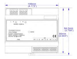
The DIN-PWS50 is a 50 watt Cresnet power supply module designed to snap onto a standard DIN Rail installation. DIN Rail mounting enables modular installation alongside Crestron DIN Rail lighting and automation control modules and other third-party DIN Rail mountable devices. All wiring connections are made using screw terminals positioned along the top and bottom, clearly accessible from the front for easy installation and servicing. Three Cresnet power ports are provided.
