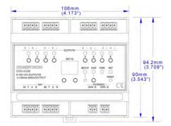
The DIN-A08 is a DIN Rail-mounted automation control module that provides eight analog output ports for interfacing with third-party lighting and heating/cooling systems.
